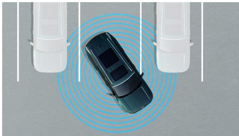
Surround View Monitor (SVM) Displays the surrounding view around the vehicle for safe parking
