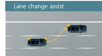
Turn signal switch initiates lane change
