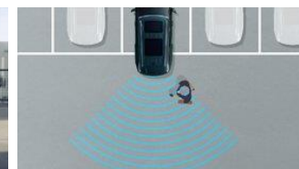
Reverse Parking Collision-Avoidance Assist (PCA-R) A safety feature that enhances reversing safety by providing alerts and braking assistance for nearby objects
