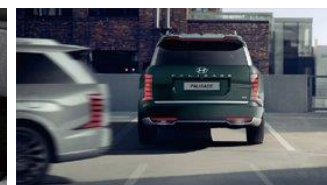
Rear Cross-Traffic Collision-Avoidance Assist (RCCA) Warns if the risk of collision with an oncoming vehicle from the left/right while reversing at low speeds is detected, and automatically assists with braking if the risk of collision increases
