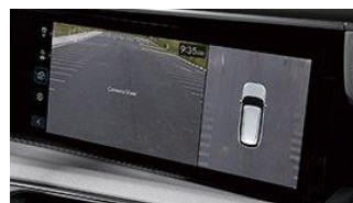
Surround View Monitor (SVM) Displays the surrounding view around the vehicle for safe parking
